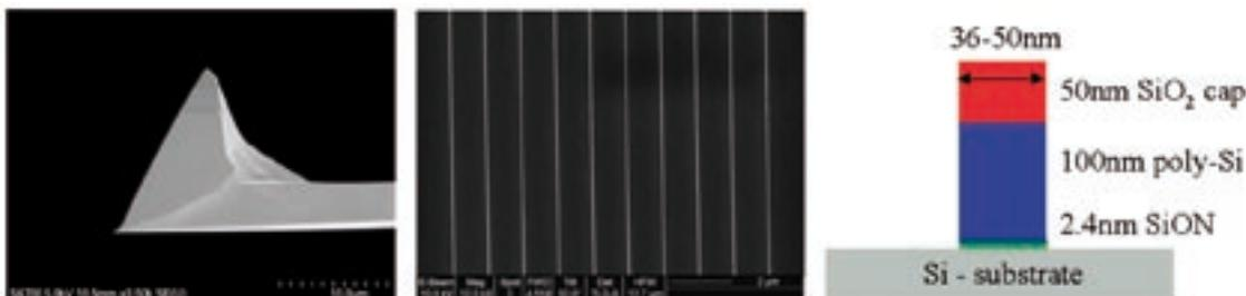
**Figure 3:** SEM picture of the type of AFM tip used for the collapsing experiments (left side) & “ASAP Line” structures under investigation as SEM picture and the principle design of the patterns on the right side
