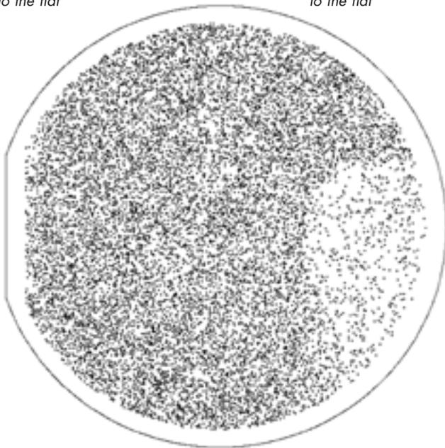
**Figure 5:** Result of the reaction of van-der-Waals bonded  $\text{Si}_3\text{N}_4$  particles with freshly prepared SC-1 (a) and SC-1 with wafer-etch products (b) ( $> 400$  nm, Surfscan 6220).
