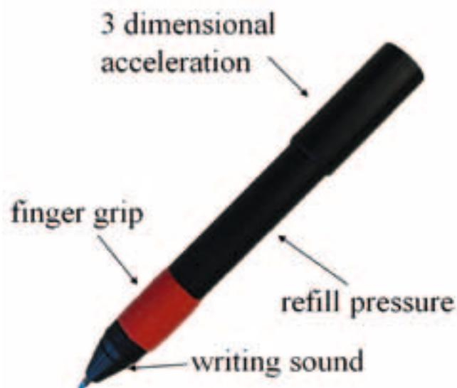
Fig. 2: sensors within the BiSP system
